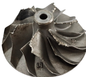
Foreign object damage to turbine wheel
