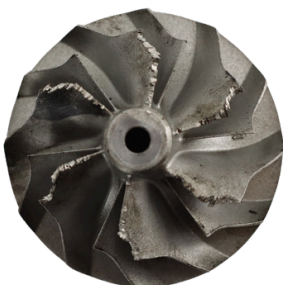
Foreign object damage to turbine wheel
