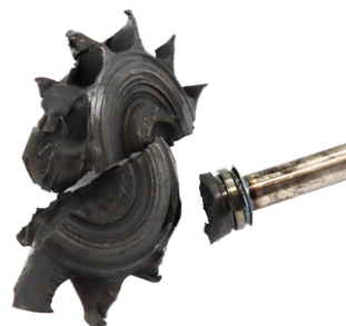
Extreme foreign object damage to impeller
