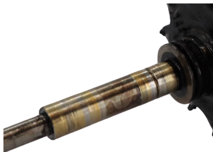
Scoring and burn marks on shaft
