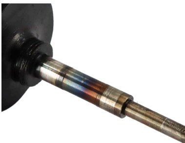
Damaged turbine shaft
