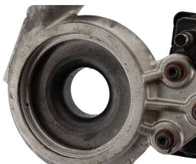
Evidence of oil leak into housing
