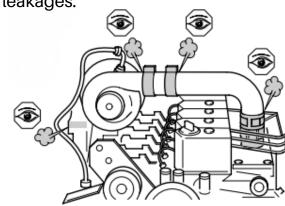
Do not leave the engine to idle for any longer than 5 minutes, as this could cause oil to escape from the turbocharger. It is essential the vehicle is road tested and the engine reaches the operating temperature.
