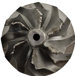
Foreign object damage to turbine wheel
