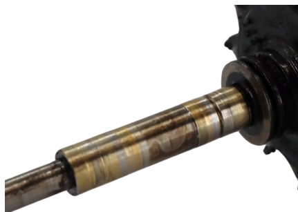
Scoring and burn marks on shaft
