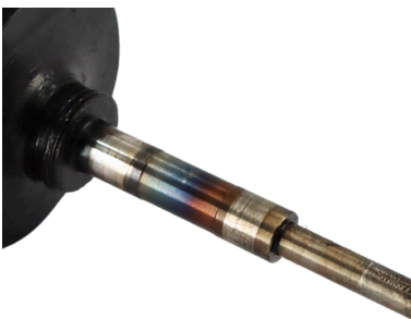
Damaged turbine shaft
