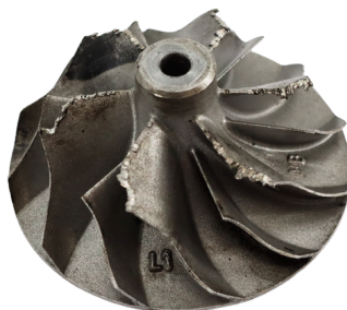
Foreign object damage to turbine wheel
