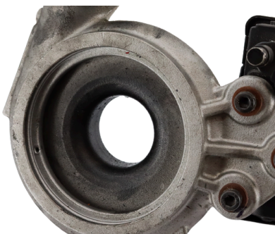
Evidence of oil leak into housing
