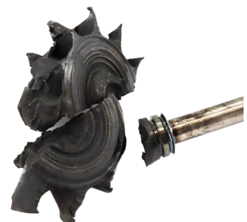
Extreme foreign object damage to impeller
