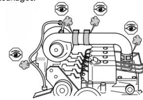
Do not leave the engine to idle for longer than 5 minutes, as this could cause oil to access the exhaust system, resulting in smoke from the exhaust.
